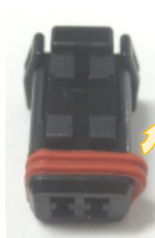
Fig.7-1 Examples for failure state of seal ring
